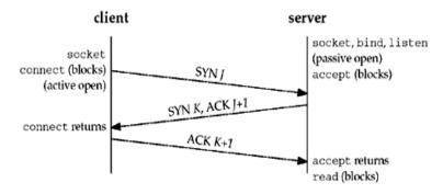
Figure 1 TCP three ways Handshake Procedure
